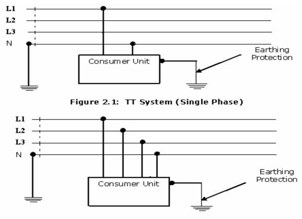
Figure 2.2: TT System (Three Phase)
