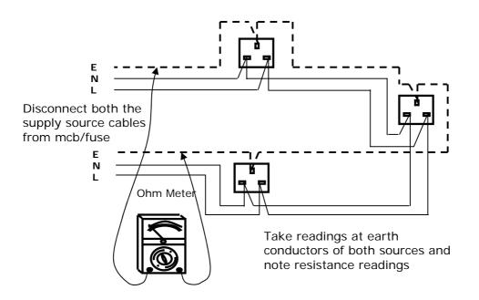
Figure 8.2 - Final Ring Circuit Conductor Continuity Test
