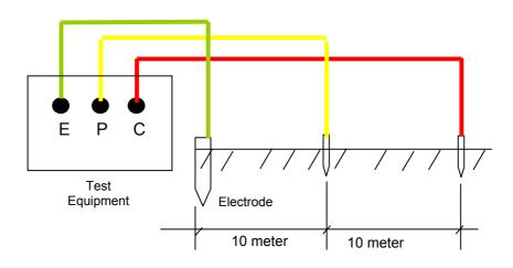
Figure 8.6 – Earth Electrode Resistance Measurement
