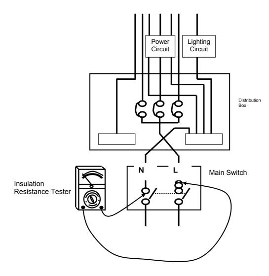
Figure 8.4 – Insulation Resistance Test
