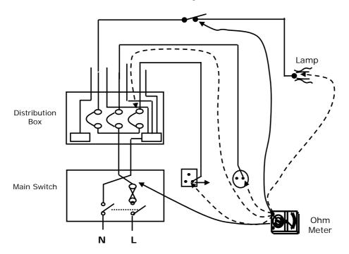
Figure 8.5 – Polarity Test
