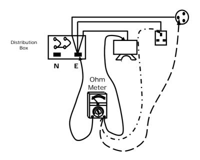
Figure 8.1 – Protection Conductor Continuity Test
