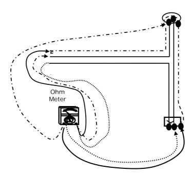
Figure 8.3 - Live and Neutral Conductor Continuity Test
