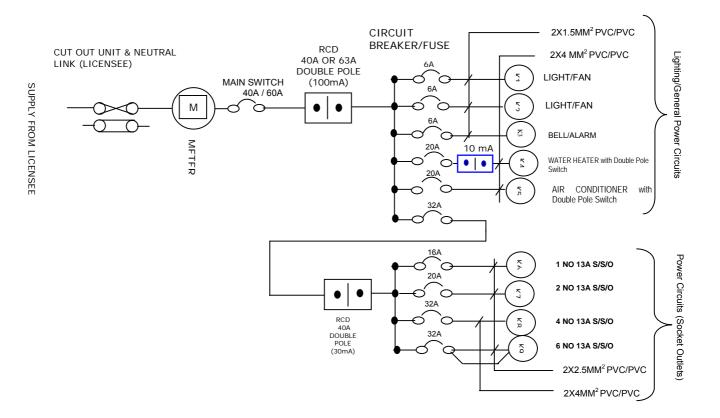
Example 3 of a single phase consumer electrical wiring is as shown in Figure 3.4
