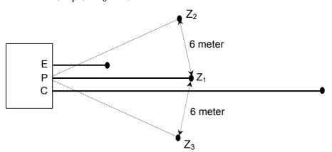
Figure 8.7: Earth Electrode Resistance Measurement
