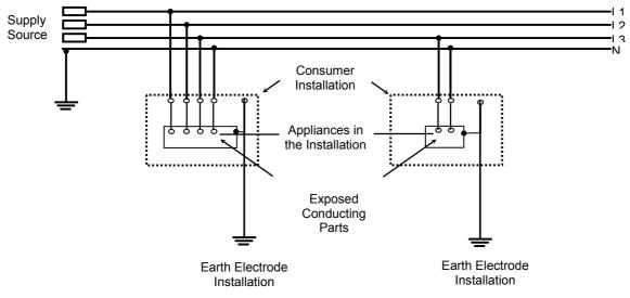
Figure 7.1: TT System Earthing
